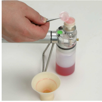
Once the entire sample has passed through the patch rinse the funnel with filtered solvent and draw through the patch. Then separate the funnel from the patch supporter and remove
