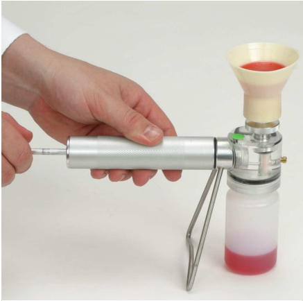
Draw the sample fluid through the patch by pulling on the vacuum pump handle. Confirm that the waste bottle and funnel-patch assembly are sealed.
