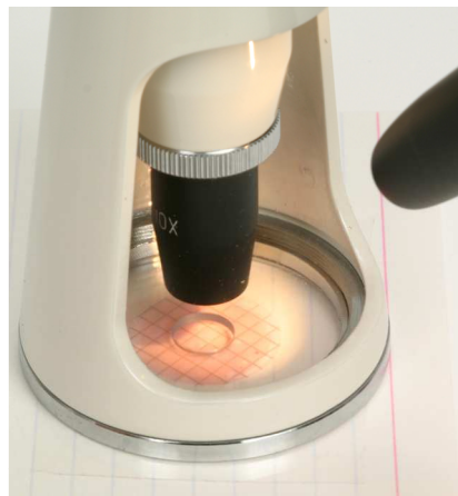
Analyze the sample with the 100x magnification field microscope. For best results hold the light source closer to the sample
