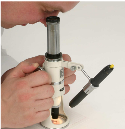
Analyze the sample with the 100x magnification field microscope. For best results in might be necessary to hold the light source closer to the sample
