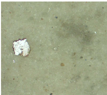
Bright metal particle typically from internal contaminant generation.
