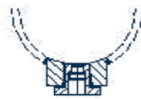
③ Contoured Half-Coupling (can also be non-contoured)
